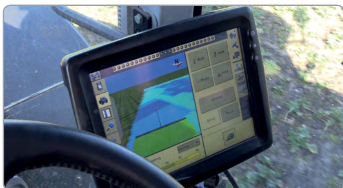
Tractor spreading fertiliser according to a variable rate application map made in CropSAT.
