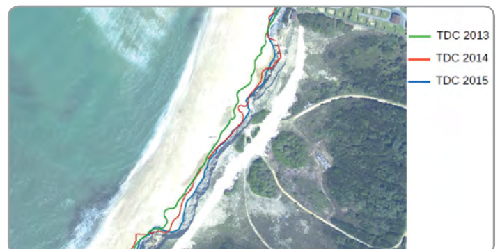
Coastline detection and change analysis from 2013 to 2015 in Pavillon Royal beach, Bidart, Basque country, south-west France.
