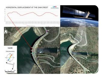
A three-year time series of displacements of a point located in the crest of the Irueña Dam, obtained with InSAR-PSI processing of Sentinel-1 image [2023].
