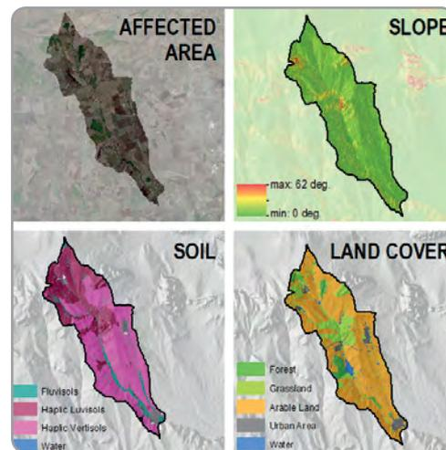
Refined watershed related characteristics information extracted from EO data is used to describe the preconditions.
