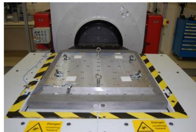
**Figure 7: CTB Mounting Hardware Attached to Fixture on Slip Table (X axis configuration)**
