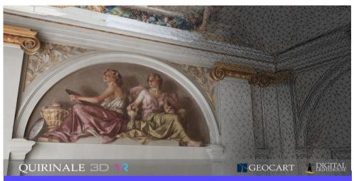
QUIRINALE 3D VR, a software for the virtual browsing of the Quirinale Palace, is the result of a prestigious project that envisaged the digital reconstruction of the rooms on the Quirinale's Main Floor (Piano Nobile) through by high-resolution laser scanners and cameras as well as advanced computer graphics techniques applied to the data collected.
