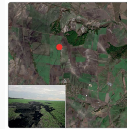
Sentinel-2 data shows not only the flooded area, but the area where the water was accumulated - thus allowing precise risk reduction measures on watershed level to be implemented.
