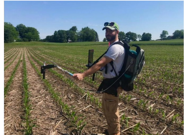
FieldSpec (ASD) Spectroradiometer reflectance collection at Maize fields at Kellogg Biological Station, MI (US)
